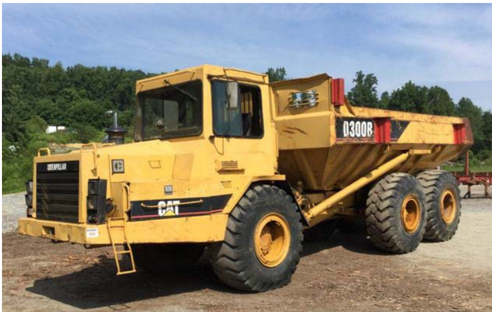
Figure TM6-6. CAT D300 articulated dump truck used for gravel hauling.
