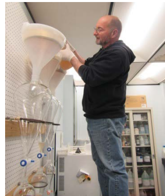
Dave Ramey filtering meat samples for evidence of trichinella .
