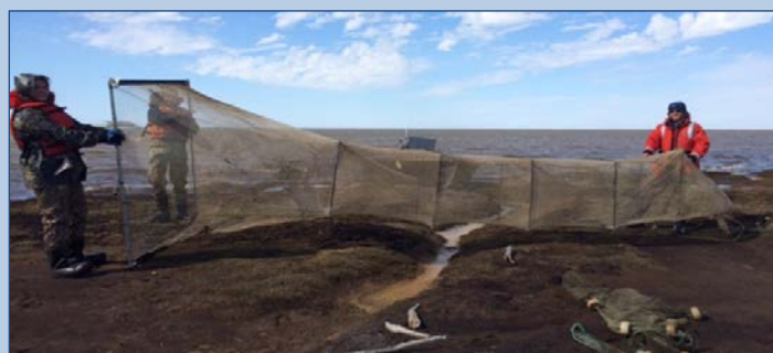
Fyke net with its funneling system of decreasing sized nets. Entrance on the left.
