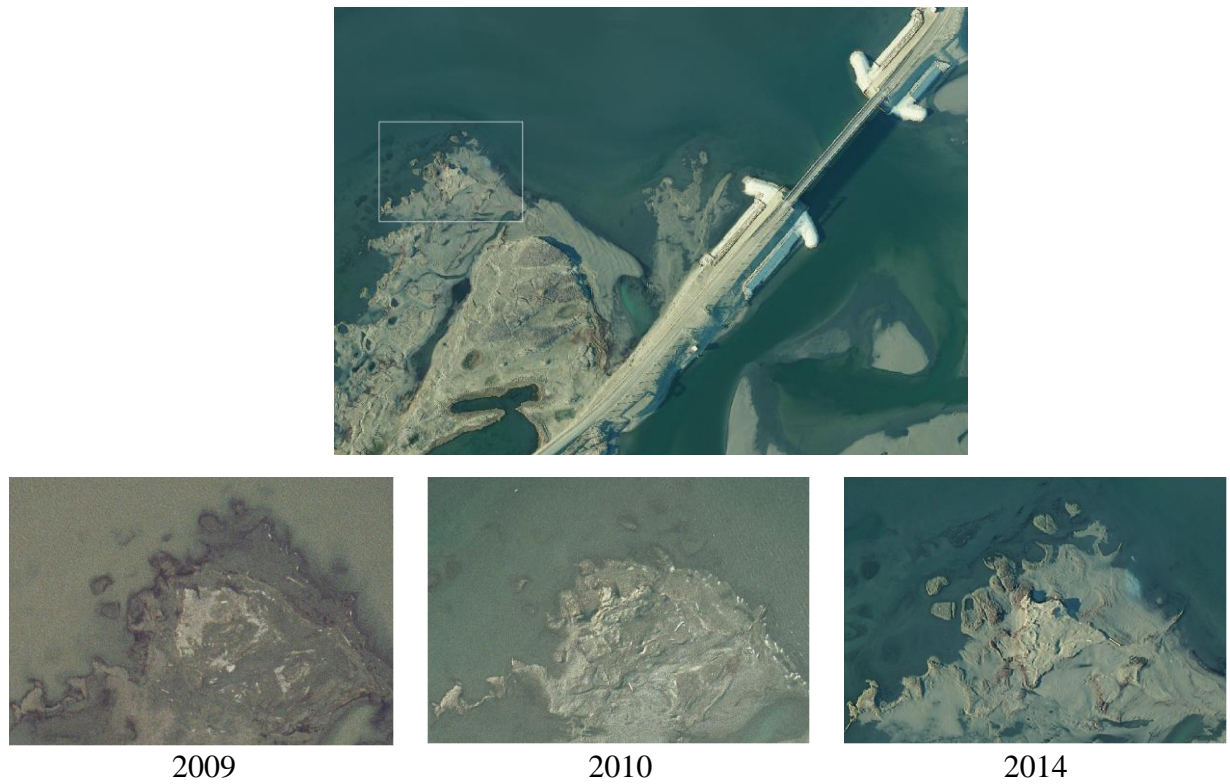
Figure 14. Example of uncertainty for shoreline interpretation on the north peninsular (marked in white rectangle) due to seasonal and tidal fluctuations when images were taken (year 2009, 2010 and 2014).
