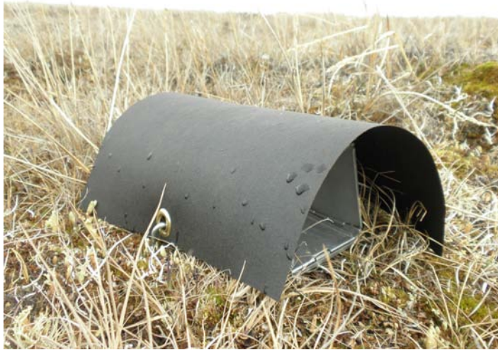
Figure 3. Folding aluminum 3"x 3.5" x 9" Sherman live trap with 12" x 12" waterproof roofing felt cover.
