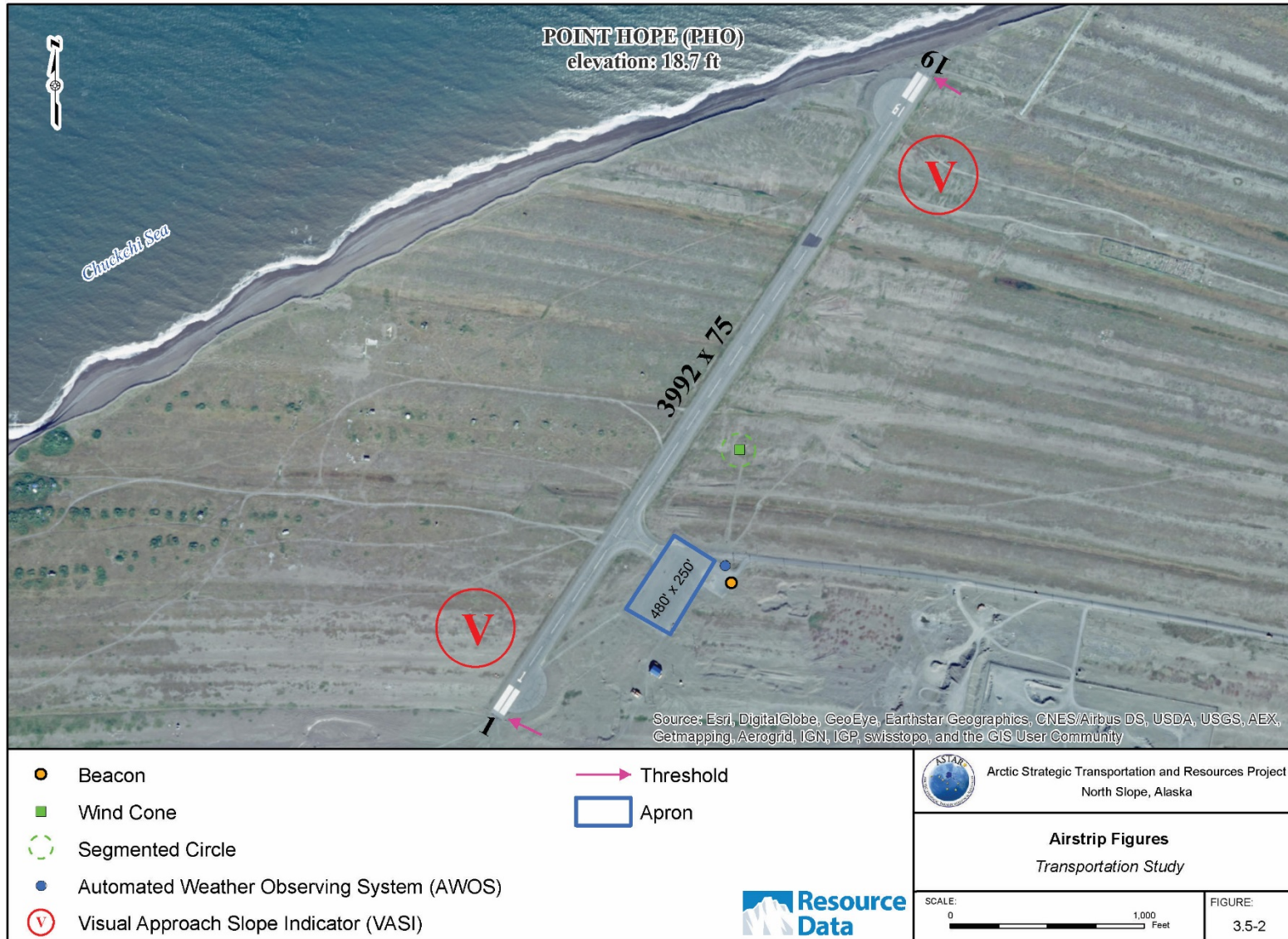
Figure 3.5-2. Point Hope Airport
