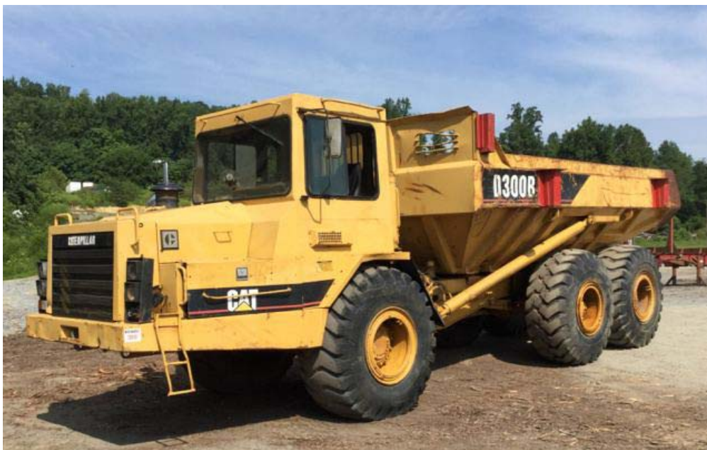
Figure TM5-5. CAT D300 articulated dump truck used for gravel hauling.
